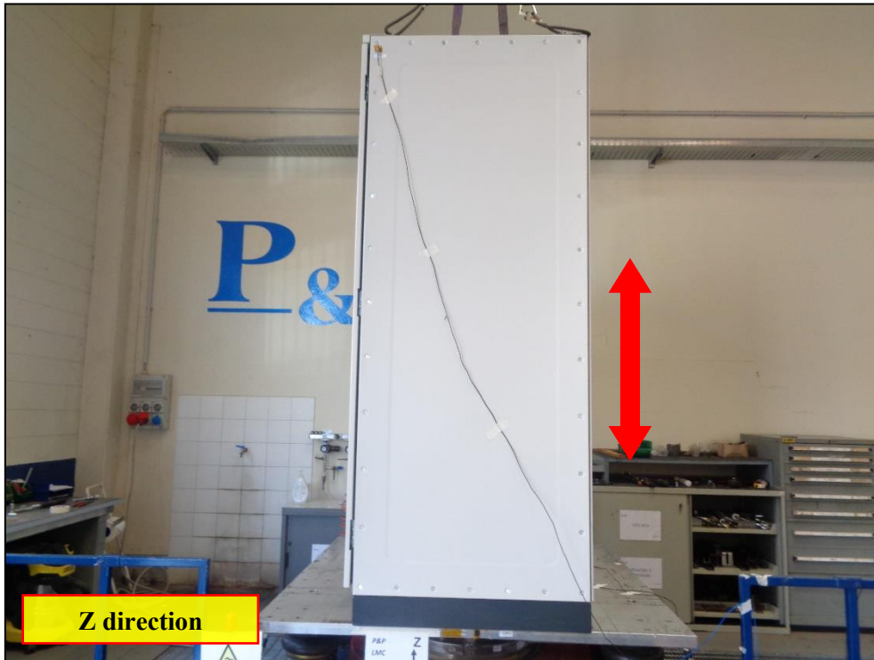
Photo 1 – Test configuration in Z direction
